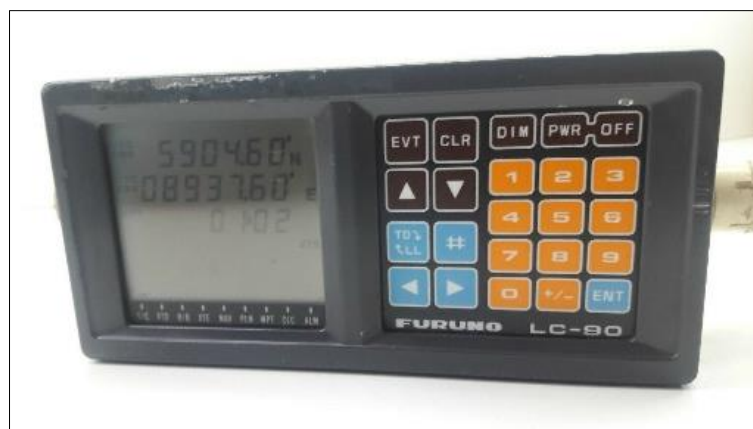
Figure 1: Example of LORAN-C Furuno receiver, extracted from [1]
