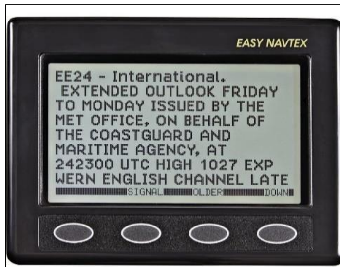
Figure 6: Example of NASA Easy NAVTEX receiver, extracted from [6]
