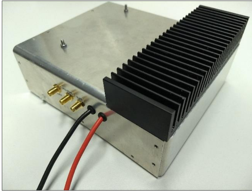
Figure 53: VDES transceiver prototype developed by EGATEL for the POLARYS project
